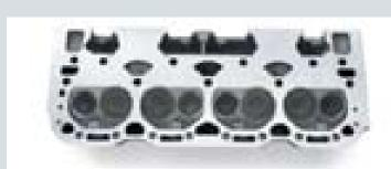
LT4 Aluminum Cylinder Head Assembly (combustion chamber)
